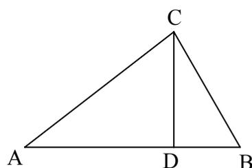
$$\begin{aligned} \overline{BC}^2 &= \overline{CD}^2 + \overline{BD}^2 = b^2 \sin^2 A + (c - b \cos A)^2 \\ &= b^2 + c^2 - 2bc \cos A \end{aligned}$$
